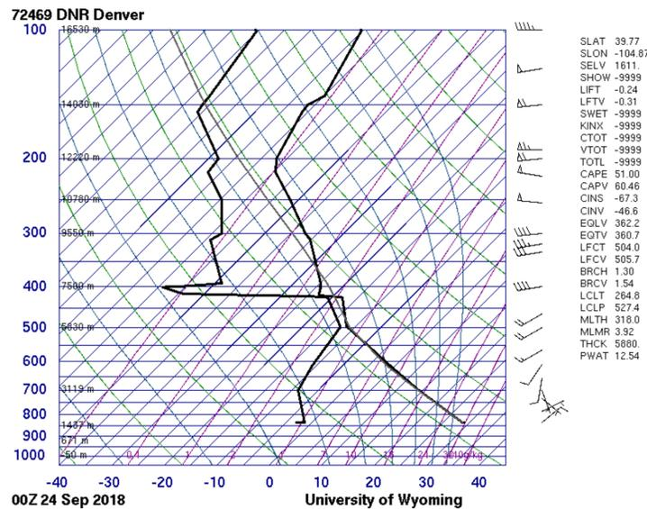
Figure 1: The Skew-T plot for September 28<sup>th</sup>, 2018 at 6:00 pm. The dark black far right line is the air temperature and the left dark black line is the dew temperature recorded by the weather balloon. [1]
