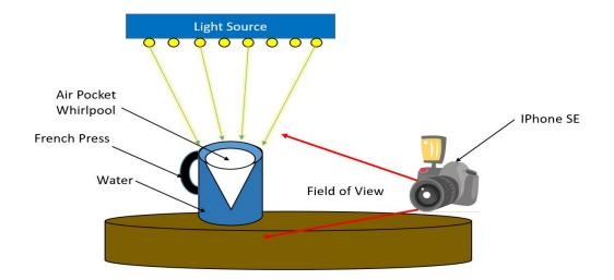
Fig 1. The apparatus set up after the spoon is removed from the french press
