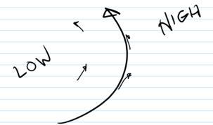
Streamlines curve because of pressure gradient. Low P is inside curve
