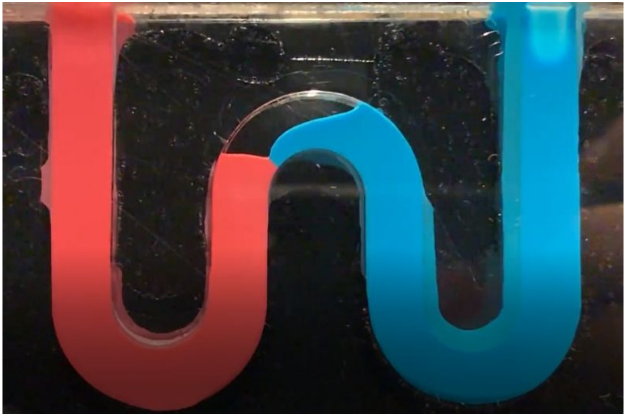
Figure 2. A snapshot of the kissing phenomenon from the video of this report. Two colored fluids of different viscosity enter the fluid until it is completely full.
