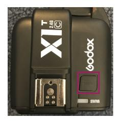
Use the button on top of the trigger to trigger the flash.
