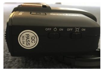
Turn both switches on the side of the trigger on.
