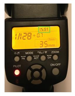
The Speedlight YN560IV flash is a different brand than the trigger we have, so sometimes there are incompatibility issues. Either use the tigger mode button to re-navigate to \$1, or turn the flash off, wait several seconds, and turn it back on again. You may have to do this more than once.
