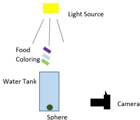
Figure 6: Picture Set Up
