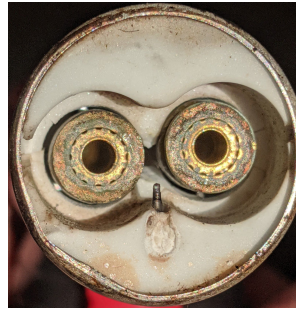
Figure 5: a picture of the torch's dual nozzles and the igniter in the center.
