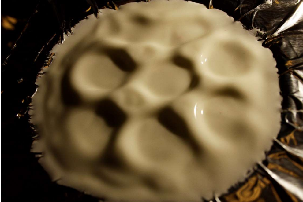
Figure 4: Dilatant being affected by sound waves
