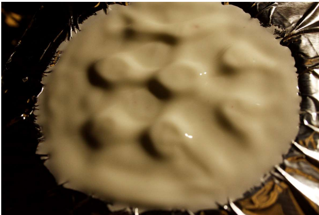
Figure 3: Dilatant being affected by sound waves
