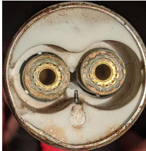
Figure-2: Nozzles on butane torch
