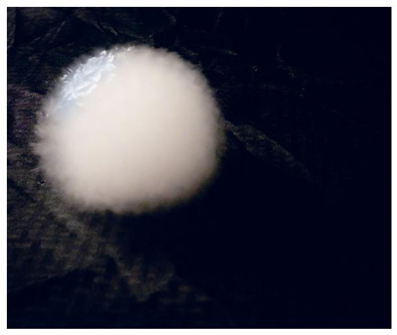
The image being analyzed in this report was taken for the first team photography assignment of the flow visualization course. The image was taken with the intent of showing the interesting fluid mechanics that occur when a bubble pops. These mechanics involved surface tension, pressure gradients and density differences resulting in expansion of the fluids inside of a bubble. The image, taken by my teammates, was that of vapor inside of a soap bubble, which I had blown, that has just been popped.
