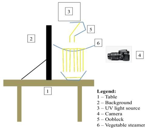
Figure 2: Setup used for imaging flow
