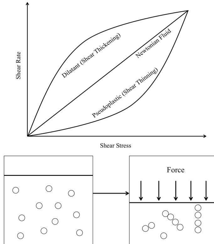
Figure 1: Differences between common types of non-Newtonian fluids (Top) and Hydrodynamic clustering (bottom)
