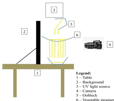
Figure 2: Setup used for imaging flow
