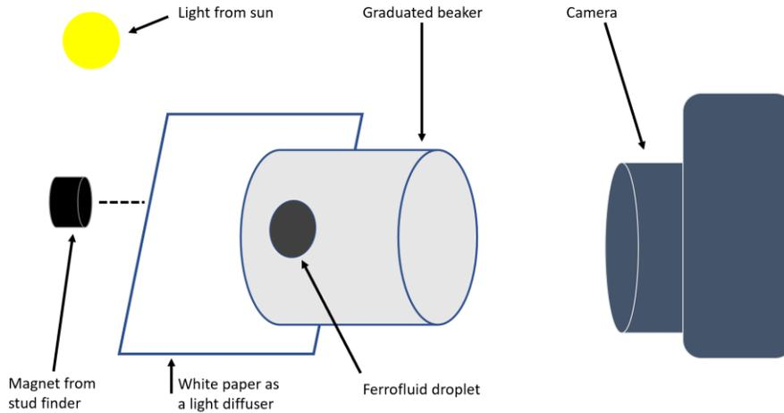
Figure 2: Diagram of experimental setup
