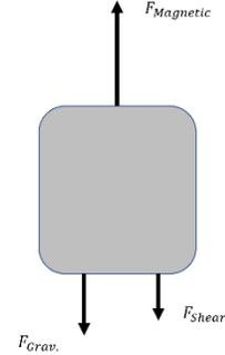
Figure 4: Fluid element free body diagram
