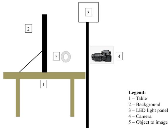
Figure 2: Setup used for imaging
