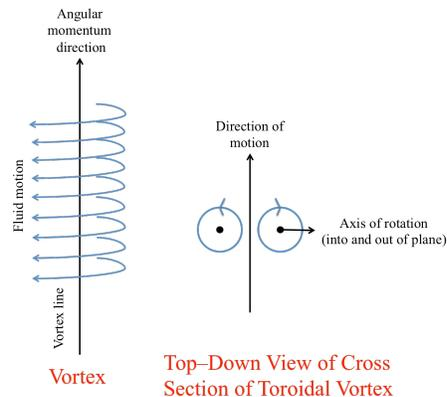
Figure 1: Motion characteristics of a Toroidal Vortex
