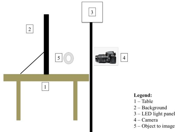
Figure 2: Setup used for imaging
