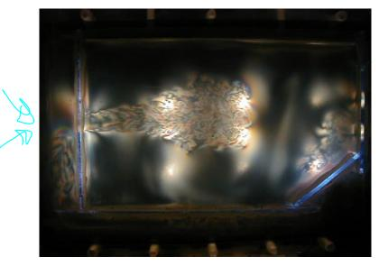
Streaming birefringence 'Blackstock fluid' has 2 indices of refraction Suspension of microscale mica flakes.
