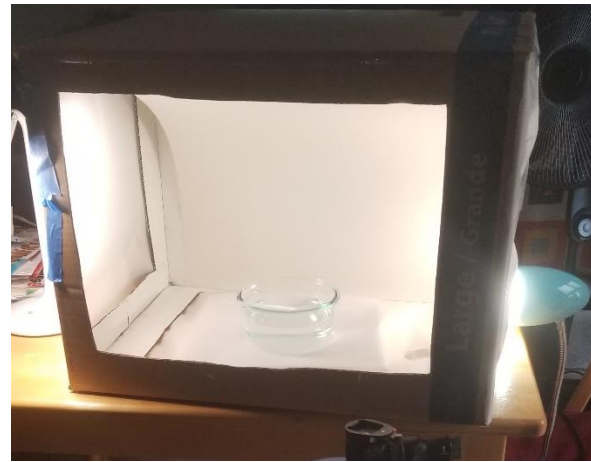
Fig. 2 (b) Light diffusion box and associated lighting
