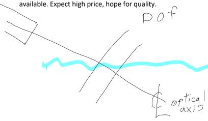
LensBaby: lets you angle the lens axis compared to the camera body axis. Effectively makes the object plane not parallel to the sensor plane. Same as 'swing' of field view camera http://lensbaby.com/lenses
