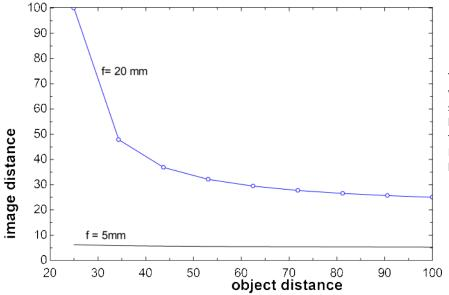
This is why small cameras with small sensors and short focal lengths have better macro capability than larger cameras. Hardly have to move the lens at all.
