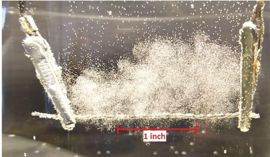
Figure 2. Approximate scale of the nucleate boiling phase.
