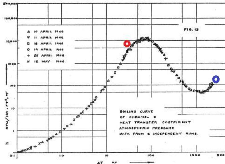
Figure 3. A figure from E.A. Farber's publication<sup>[3]</sup> showing his experimental boiling curve for water. A red and blue point have been added to demonstrate the approximate regions for the first and second video clips, respectively.
