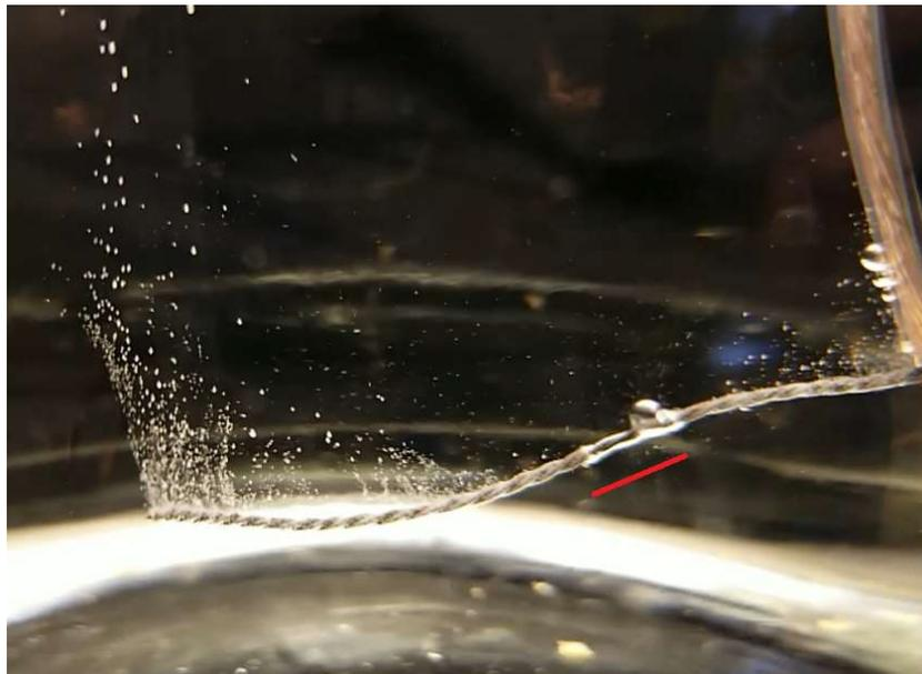
Figure 4. The length of the film boiling regime underlined in red on the cooling wire.
