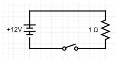
Figure 1. A circuit schematic depicting the Kanthal as a resistor connected to the voltage source. One of the battery terminals was able to be connected / disconnected as a switch.
