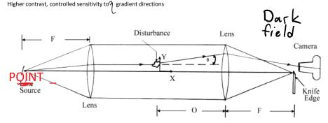
Figure 3. Schlieren System with a Small Disturbance
