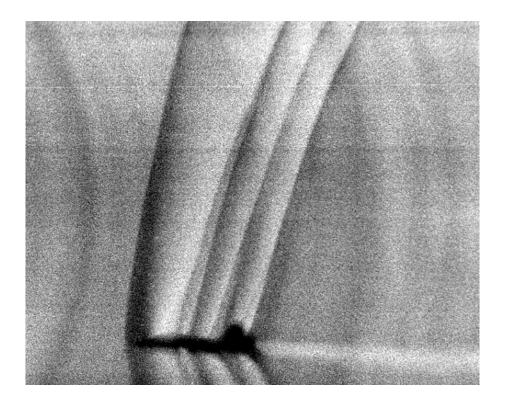
Pasted from <a href="http://commons.wikimedia.org/wiki/File:Schlieren">http://commons.wikimedia.org/wiki/File:Schlieren</a> photograph of T-38 shock wayes.ing
