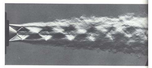
168. Supersonic jet becoming turbulent. At a Mach number of  $1.8~\rm a$  slightly over-expanded round jet of air adjusts to the ambient air through a succession of oblique
