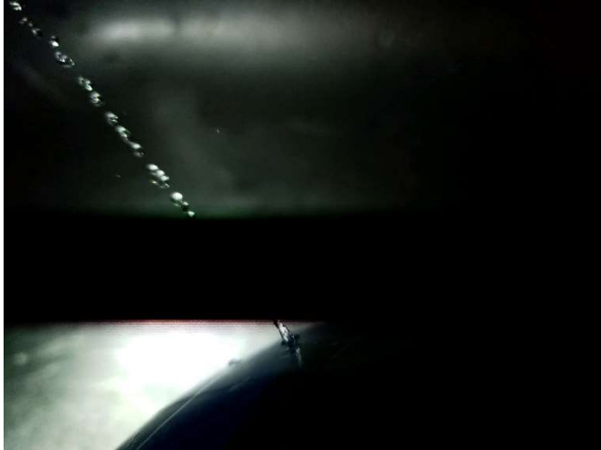
Figure 2 Image showing the black bar that results from the duty cycle of the flashlight.
