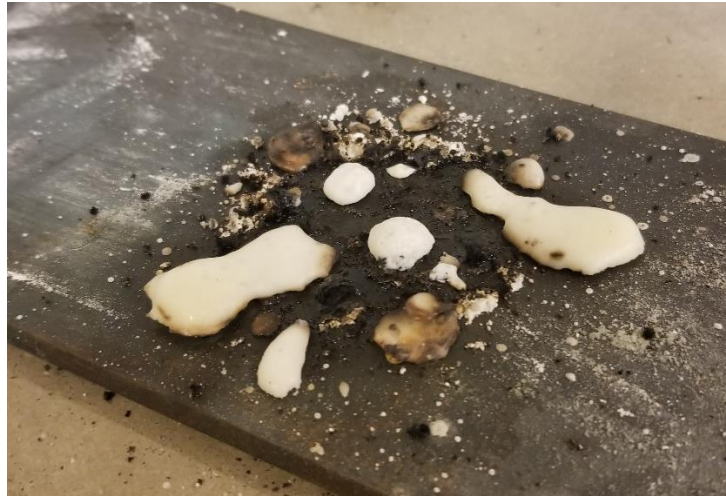
Figure 2. Chips resulting from the fuel combustion. As with the orbs, they are likely potassium carbonate, possibly with some concentration of potassium hydroxide.
