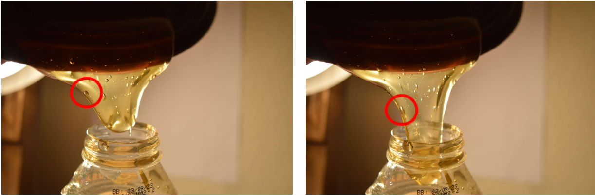
Figure 4. Two comparison frames to determine velocity of the honey.
