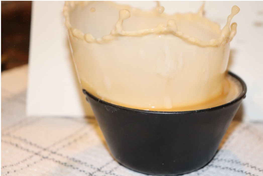
Figure 2. Full unedited image of the non-Newtonian fluid and rock impact.
