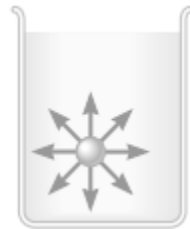
Figure 1 - Forces on a sphere of oil in water [2]
