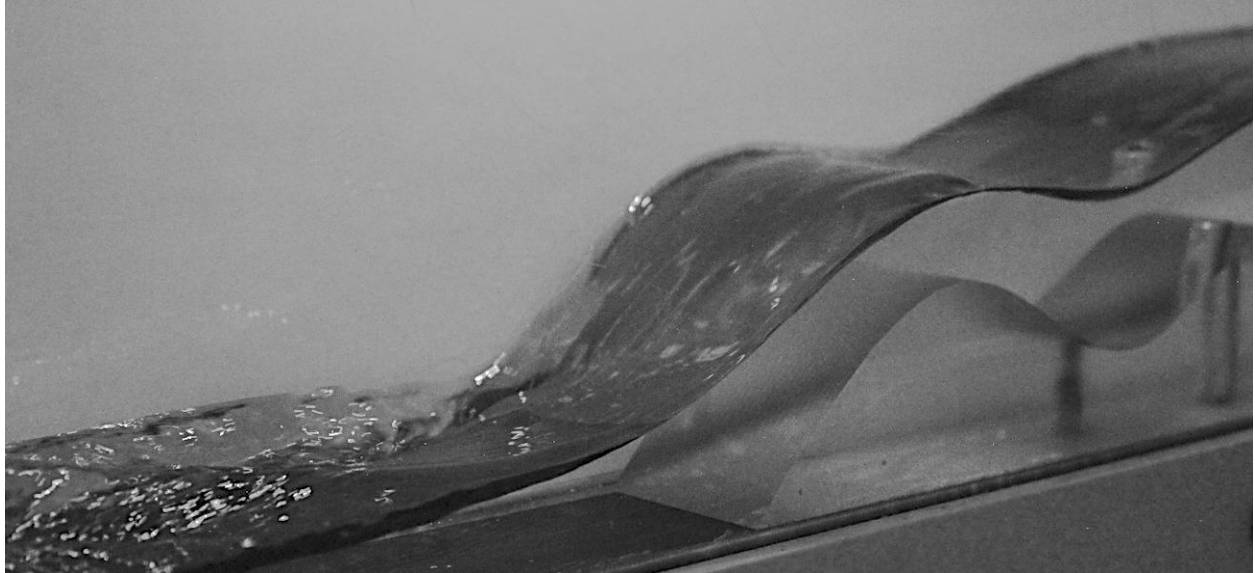
Figure 1, Depiction of the Flow Phenomenon of water in open channel flow over two hydraulic jumps, flowing from right to left
