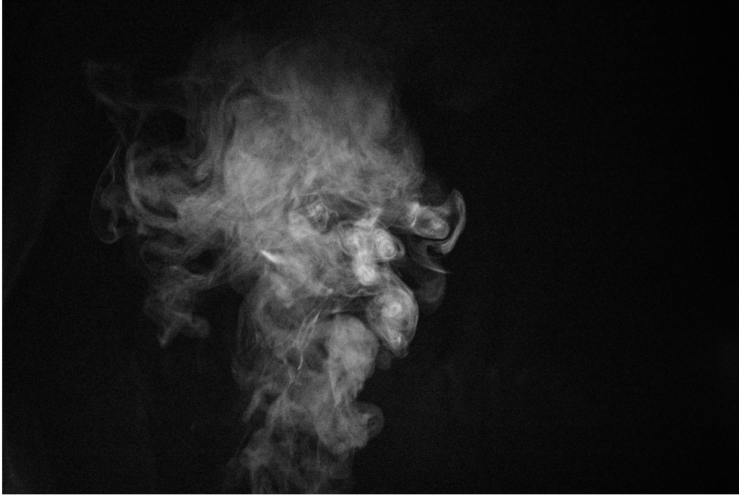
Figure 1: Visualization of Turbulence Using Fog Machine
