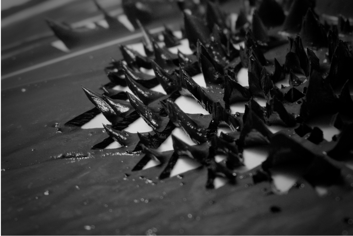
Figure 1: Magnetorheological Fluid Experiencing Magnetic Field
