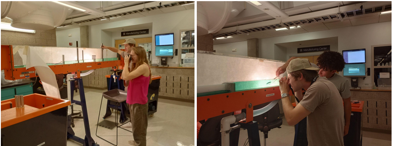
Using the flume to create open channel flow and observe obstruction in stream
