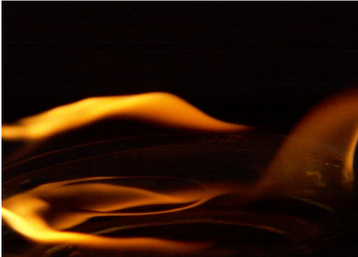
Figure 1: One frame from the video showing the initial flame ignition. This image also shows the boundary layer between the lighter fluid and the water it is floating on which will be discussed later.
