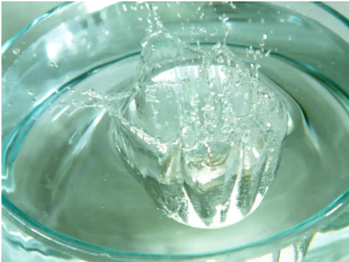
Figure 1: One frame from the video showing the cavity created by a dropped golf ball
