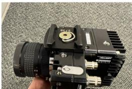
4. Take the Phantom power supply and the ethernet cable and attach them to the camera.
