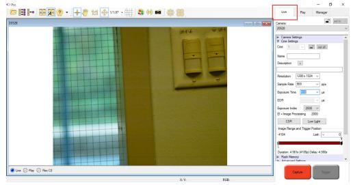
8. Change the settings of the camera according to your needs. (Lower resolution will allow taking a higher frame per second videos. The highest frames per second for each resolution can be found when clicking the sample rate tab for each resolution). Exposure time can be set according to the light available in the set. The amount of time that can be recorded is shown below the image range and trigger position bar.
