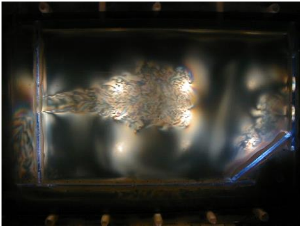
Streaming birefringence 'Blackstock fluid' has 2 indices of refraction Suspension of microscale mica flakes.
