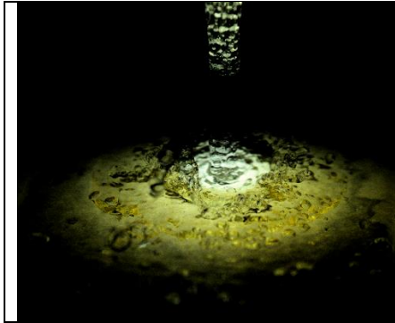
Figure 3: Water jet flowing over honey, after initial impact, the jet formed and collapsed a pocket in the honey and began to flow over the honey more smoothly.
