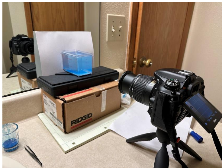
Image of the testing setup with the Nikon D7500 on a tripod.
