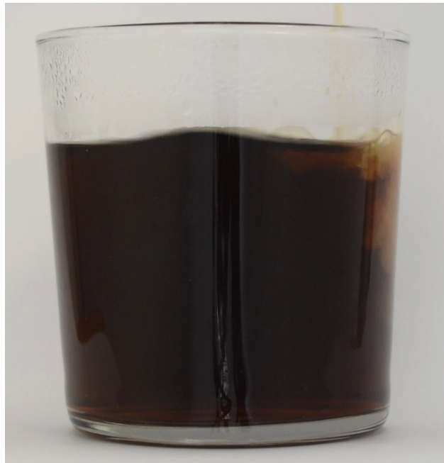
Figure 2: Disturbance wave on surface of coffee from initial impact of the oat milk.
