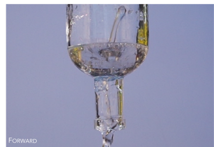
Figure 3: A jet forms on the surface of the mineral oil/water mixture.
