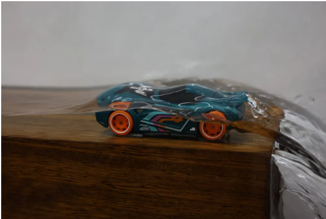
Figure 1: Water breaking over a blue Hot Wheels car as it travels down a water flume.
