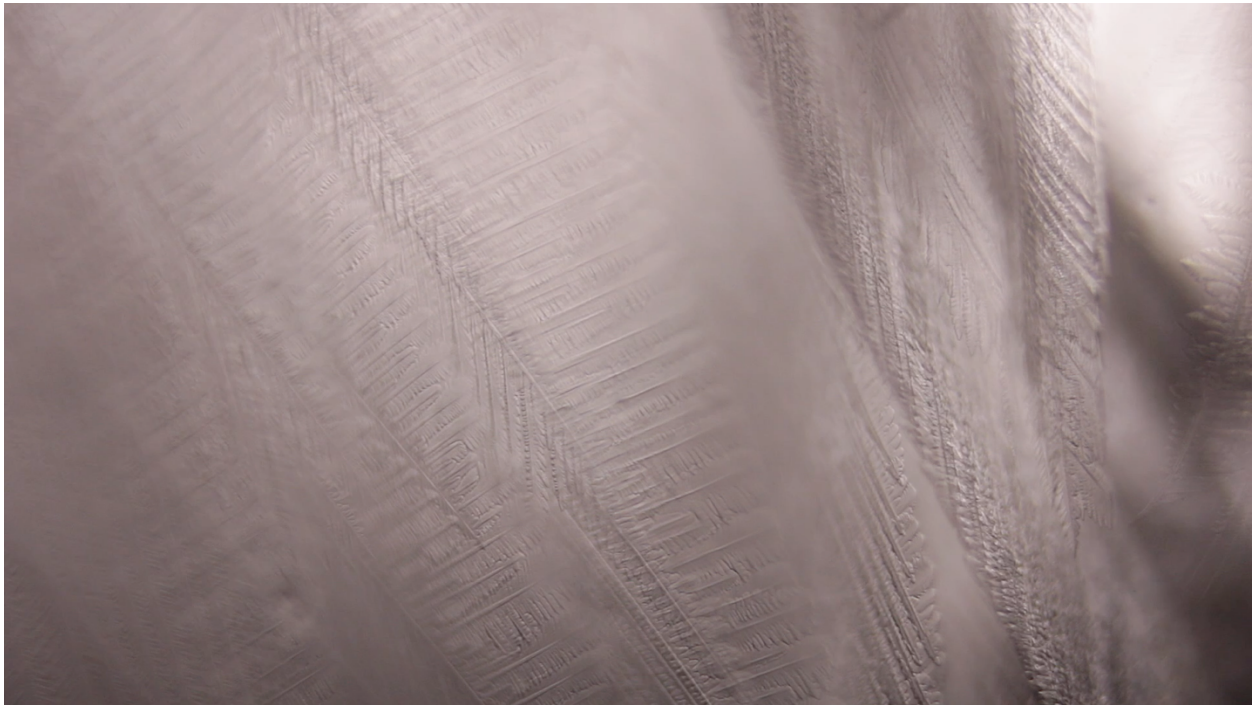
Figure 2 Planar dendritic crystallization as seen in bottle supercooled to -2.8°C
