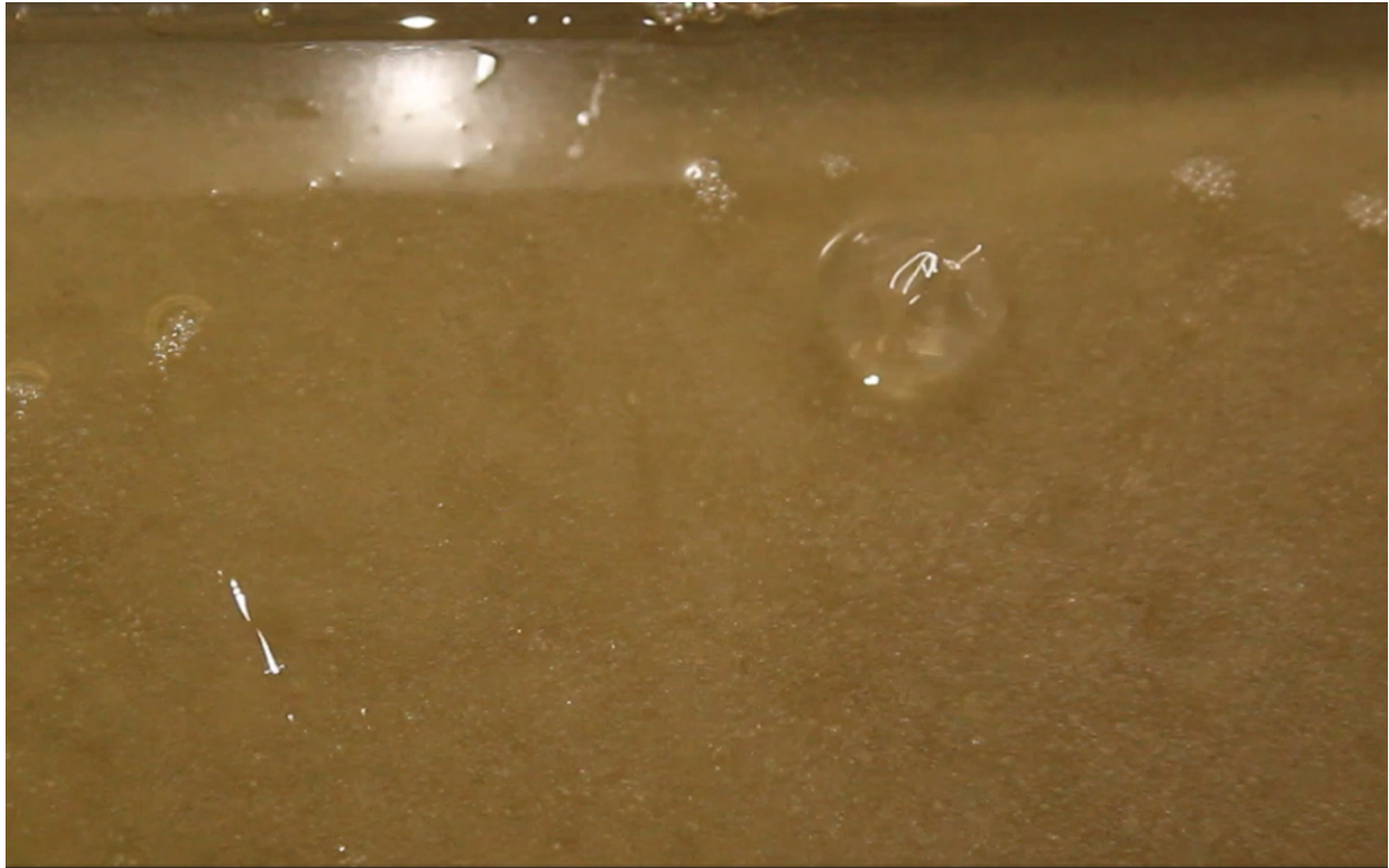
Figure 2: A screenshot of the moment a big bubble burst when we added droplets of water to the experiment setup showing the mica powder moving around
