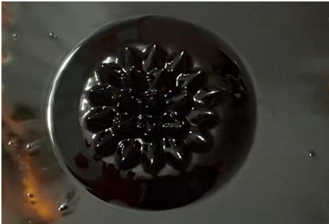
Figure 3: Snapshot of a ferrofluid's Normal Field instability with white lighting
