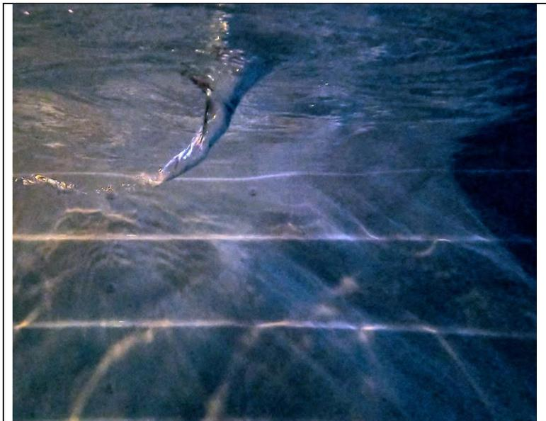
Figure 4: Vortex in the wake of a kayak paddle, the narrowest point of the vortex funnel trails after the paddle in its path.
