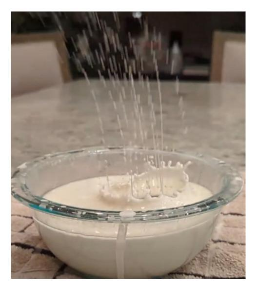
The video was taken for the Team Third assignment for Flow Visualization. The goal of this assignment was to use your team as a resource when capturing some type of flow phenomenon. The purpose of this video was to show the flow of a more dense liquid by adding cornstarch to water.
