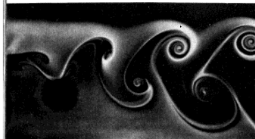
94. Kármán vortex street behind a circular cylinder at R=140 . Water is flowing at 1.4 cm/s past a cylinder of diameter 1 cm. Integrated streaklines are shown by electrolytic precipitation of a white colloidal smoke, illuminated
