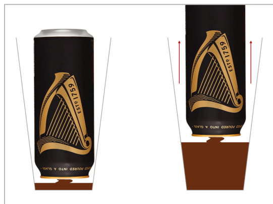
Figure 2: Flow apparatus sketch showing the proximity of the can to the liquid level when pouring the pint
