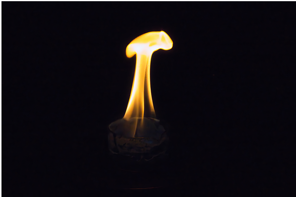
Figure 4: Puffing and necking dynamics of plume
