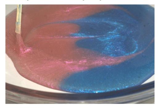
The tapered shape of the mixing shows how viscous forces drag the syrup behind the stir stick. The stir stick was moved relatively slowly at about 1 revolution in 5 seconds with about a 5 cm radius. This gives a velocity of 0.01 m/sec. For the characteristic length, 1 cm is used as that was the approximate thickness of the pool of corn syrup. The Reynolds number is the most useful nondimensional number in understanding the forces at play in this mixing:
