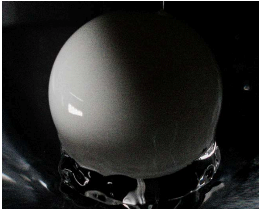
Figure 3: Moment just as surface tension breaks around a rapidly surfacing object
