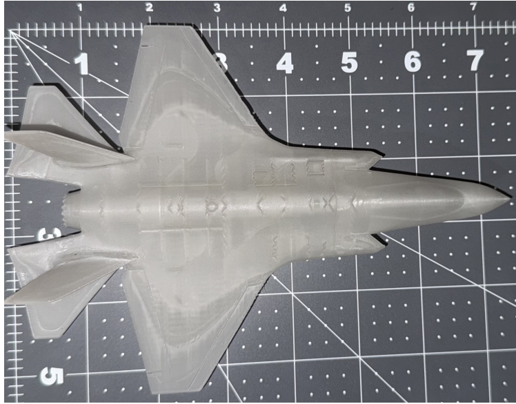
Figure 4: 3D Printed delta model in glow PLA
