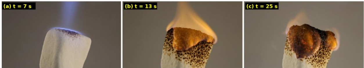
Figure 2. Frames from the video: (a) the torch jet striking the top face, (b) the marshmallow's own flame once the torch is gone, and (c) the blistered, charring surface beneath a shrinking flame.
