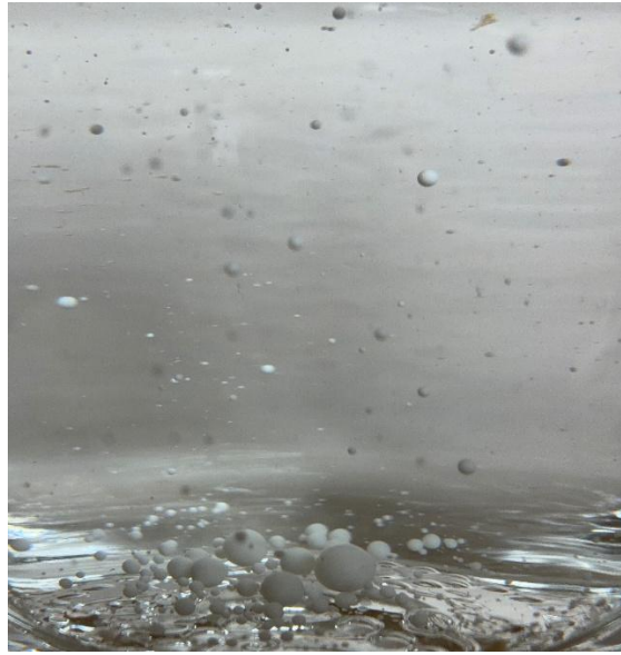
Figure 3: Image of molten wax forming spheres when surrounded by water.
