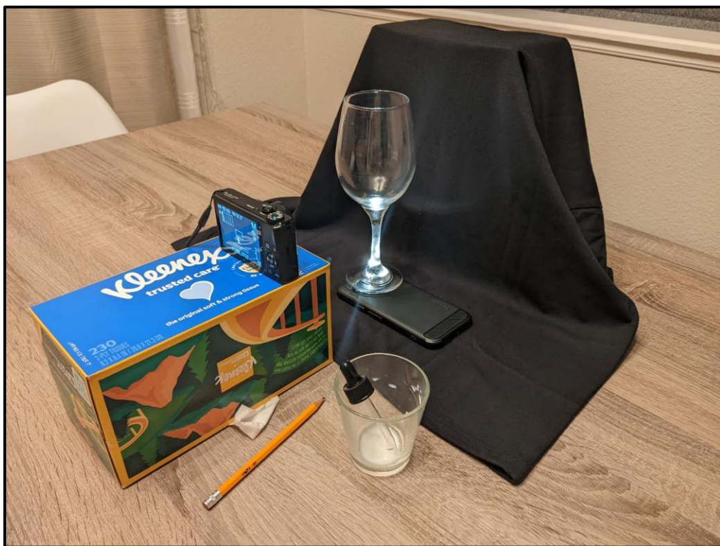
Figure 1: The experimental setup showcasing the wine glass standing on the phone flashlight, the dark backdrop, and the camera position.
